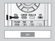
You can freeze the picture when watching a television programme simply by pressing the "STILL" button. To return to normal viewing, press it again.
